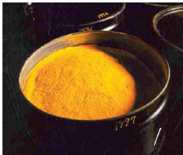
The end result of uranium milling is a dry, yellow powder known as yellowcake.
