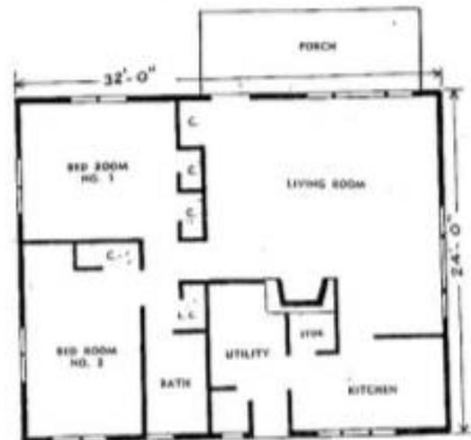
**INTERIOR PARTITIONS** Partitions and ceilings are painted gypsum board over wood studs. Bathroom walls are finished with glazed wallboard.
