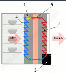
The heat from inside the refrigerator is transferred to the coils and is then sent outside of the refrigerator. The food in the refrigerator stays cold and the back of the refrigerator is warm.
