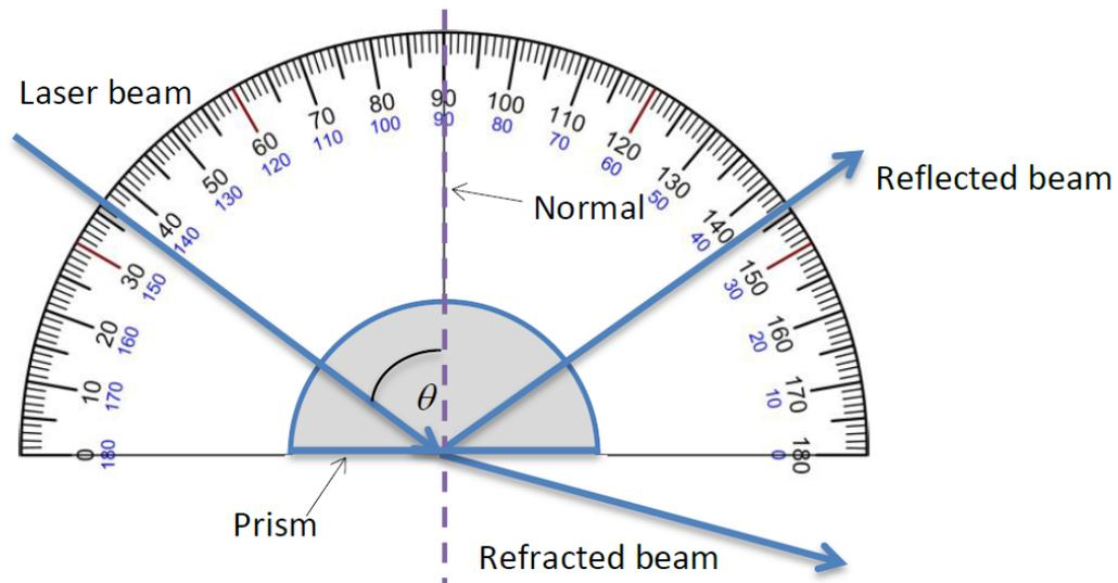
The students move the laser, maintaining the beam along a radius. They will find that for large values of  $\theta$ , 100% of the light will be reflected off of the flat surface of the semicircle, and the refracted beam completely disappears. The smallest angle  $\theta$  at which total reflection occurs is called the critical angle of incidence.
