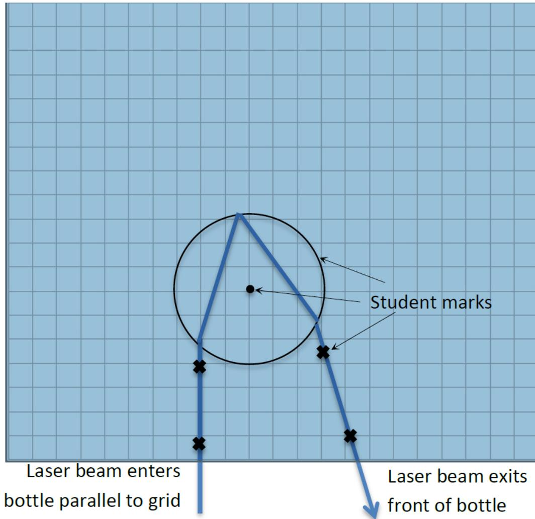
Students then analyze their data by removing the bottle, drawing lines through the points they previously marked, and measuring the angle  $\theta$  between their entering and exiting beam. They also measure the shortest distance  $d$  between the entering beam and the center of the circle by measured along a grid line. An example appears below:
