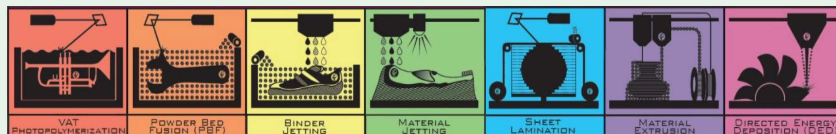
Figure 1: Simple visual description of each type of additive manufacturing. From left to right is Figure 1a, 1b, 1c, 1d, 1e, 1f, 1g. (Diagrams courtesy of Hybrid Manufacturing Technologies)
