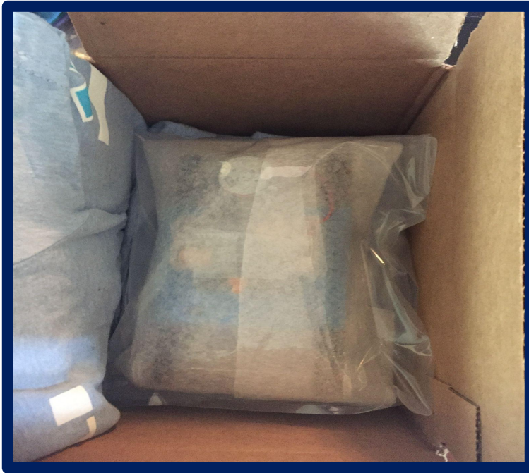
Packaging Design 4: Method 30 enclosed whole tank. Non-military void filler. A-A 59135 cushioning wrap
