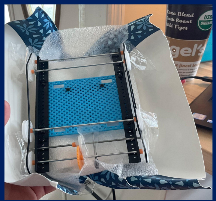
Packaging Design 2: Method 10 with blocking using paper plates. Disassembly of object for packaging
