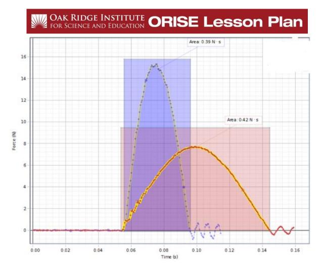
Note that the golf ball clearly has a smaller impact time and experiences a larger peak force (~15N vs. ~7.5N) then the tennis ball. For an ideal bumper or helmet design, the ideal impulse curve is "fattened" by having a very large time of impact and small peak force exerted.
