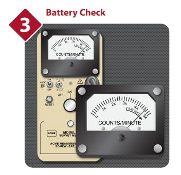
Turn instrument on and perform battery check. Replace as needed.
