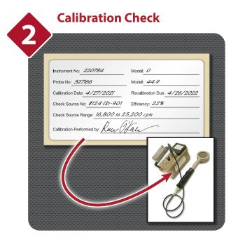
Verify instrument is within the recalibration date. (typically 1 year from calibration date).
