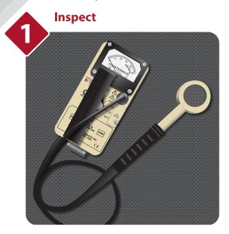
Inspect for damage, connect cables, install batteries.
